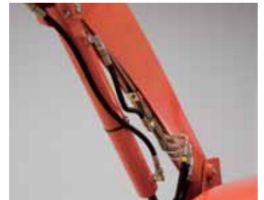
Protected Cylinder Tubes
